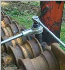
Torque multiplier used on tracks
