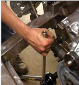
Torque multiplier used in inaccessible areas
