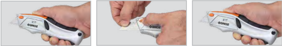
Squeeze lever to load blade Quick release button to slide out used blade Squeeze lever again to load new blade
