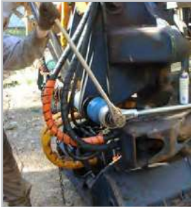
Torque multiplier used for machine nut tightening
