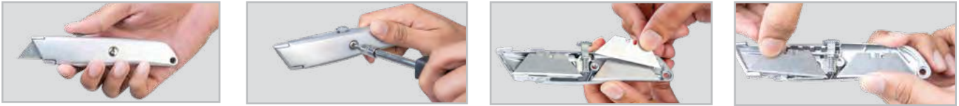
Press the lever down & push forward to load blade Open screw to reach blade storage compartment Quick & convenient blade interchange Total 5 blades: 4 blades come as spare inside the knife, with 1 blade in use
