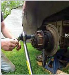
Torque multiplier used for lug nuts
