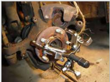
3 Jaw Puller used for removing tyre hub
