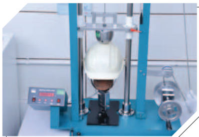
SHOCK ABSORPTION TEST
