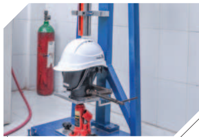
PENETRATION RESISTANCE TEST
