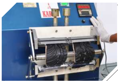
SOLE FLEXING RESISTANCE TEST
