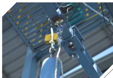
DYNAMIC STRENGTH TEST TYPE A ANCHOR
