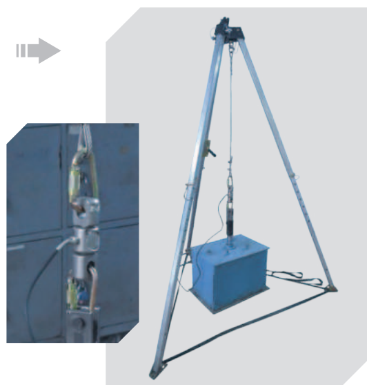
STATIC TEST OF TRIPOD
