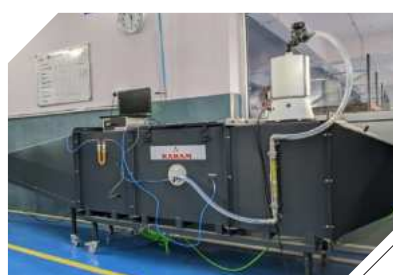
DOLOMITE DUST CLOGGING TEST
