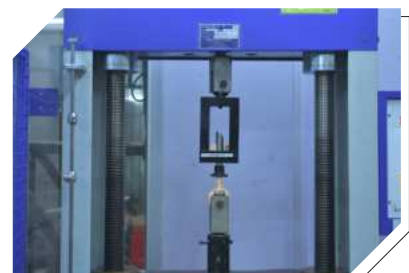
STATIC TEST OF TYPE B ANCHOR
