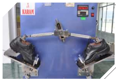
SHOE FLEXING RESISTANCE TEST
