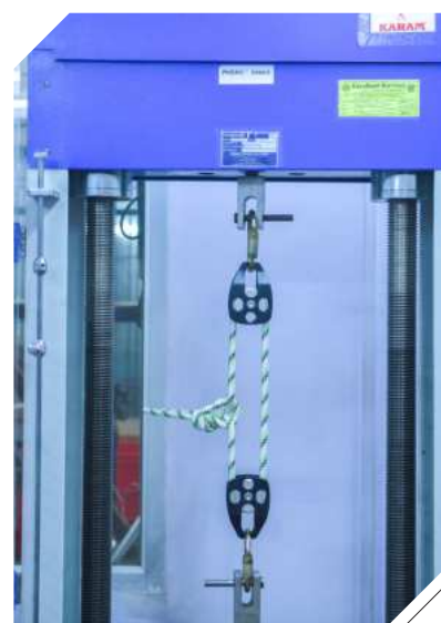
STATIC TEST OF PULLEY
