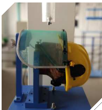
PENETRATION RESISTANCE TEST
